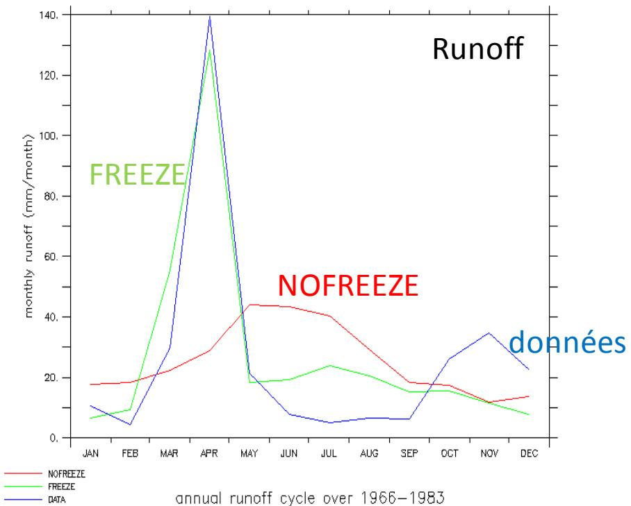
Mean annual cycle of soil temperature at 20 cm (a) and of overland flow (b) simulated at Valdai (Russia) over 18 yrs. Atmospheric forcing and field data were provided in the framework of the PILPS 2d experiment (Schlosser et al., 1997). Red and green curves respectively refer to the model without and with the soil freezing scheme; the blue curve represents the data.
