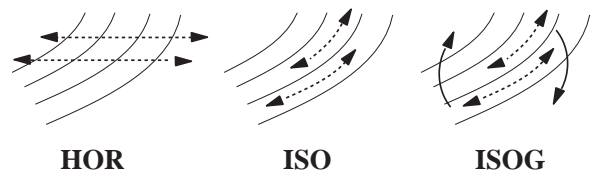
FIG. 1. The 3 lateral diffusion parameterisations used in this study. HOR horizontal diffusion, ISO isopycnal diffusion and ISOG isopycnal diffusion plus eddy-induced velocity (see text). Isocontours represent the neutral density field.
